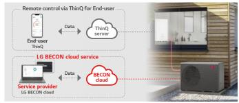
With ThinQ, users can regulate the temperature and operation mode of the R290 Monobloc anytime, anywhere. Additionally, the BECON cloud enables installers or service partners to provide remote monitoring, servicing, and firmware upgrades
